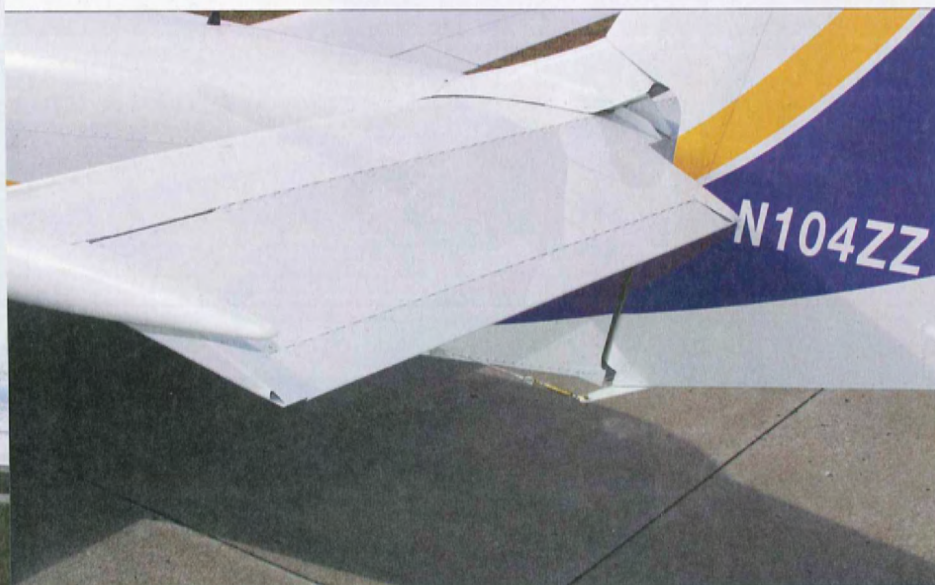
A near-full-span trimtab graces the left elevator. Simple sheet-metal surfaces are meant to be as light and easy to assemble as possible.
