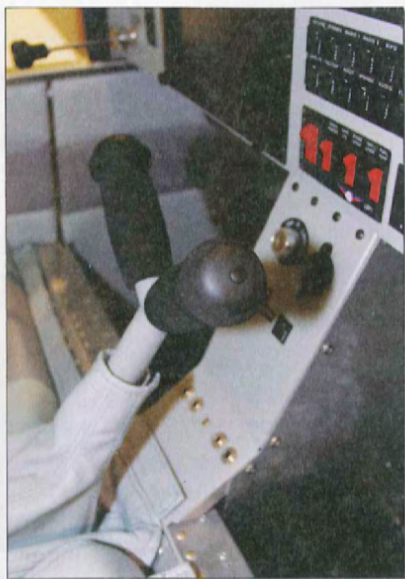
One stick for two. Zenith's uncommon Y-shaped control stick gives both occupants a shot at the landing.
