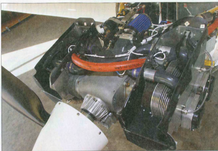
A top-down induction system is fed fuel through electronic fuel injectors. The air-cooled heads have sufficient fin area to keep the engine cool even at low indicated airspeed.
