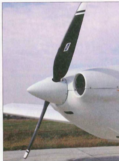
Electronic fuel injection means there's no carb to spoil the cowling's clean lines.
