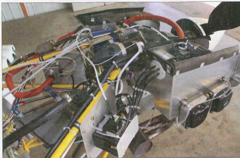
The low installed weight of the UL Power 350iS dictates a long engine mount. In the foreground is one of the two coil packs.
