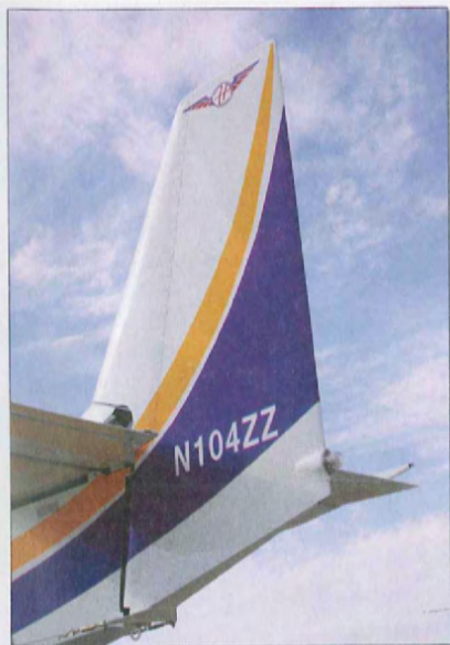
Blink and you'll miss it. Zenith gave the 650's rudder more sweep than the 601's for a modern look.
