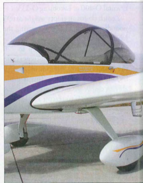
New for the CH 650 B is a canopy that provides excellent visibility even for tall pilots.
