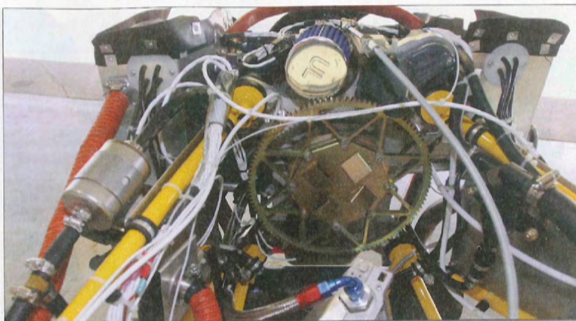
Inside the gold-anodized flywheel/starter-gear assembly is a motorcycle-style, permanent-magnet alternator rated for 30 amps.
