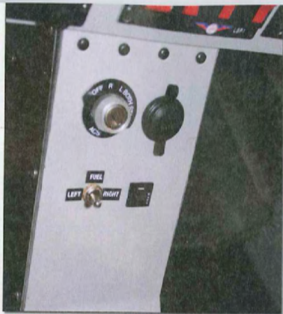
The UL Power's injection system called for electric fuel-tank switching in the 650.
