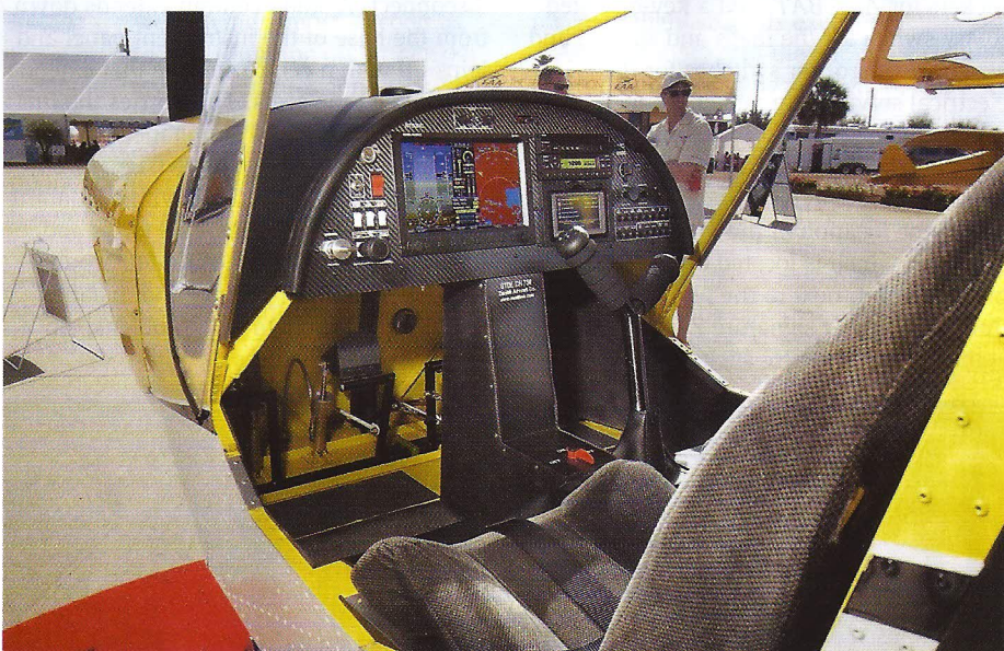
Below right: one further bit of characteristic Heinz functional design – the Y-shaped central stick is shared between PIC and passenger/co-pilot. Simple but effective...
