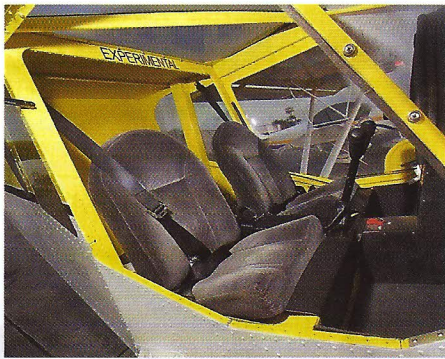
Above: adjustment of standard seats requires a spanner. Sliding seats are an extra-cost option
