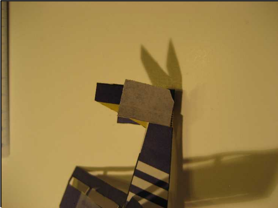
Bending up the horizontal stabilizer
